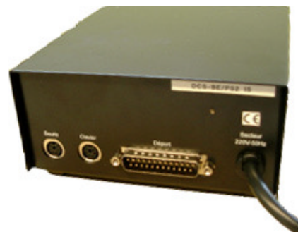
Metallic box enclosure
